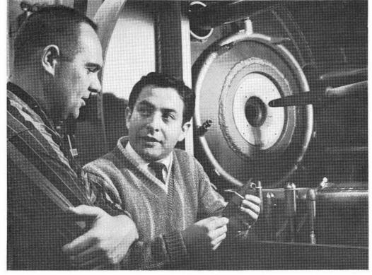
PLASMA JET test of an ASP generator design shows glowing emitter portion at the front of the nose cone and cooler collector section at the rear. Also visible is the shock wave in the plasma stream which is entering the test chamber from the right. Emitter and collector areas are connected by an internal rod through the separating insulator which completes a load circuit. Up to 30 amps of power per sq. in. of emitter surface is created during reentry.
